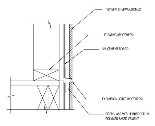
NOTE: All joints of cement board must be treated with 4" fiberglass mesh embedded in polymer based cement.
